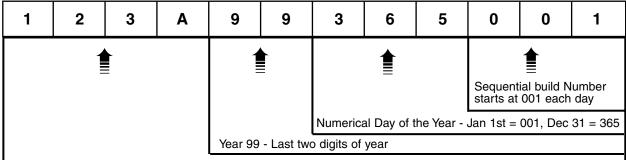
First Digits indicate model, example shown is a 123A Glassfront Merchandiser - The machine identification may contain up to six characters dependent upon the model.
