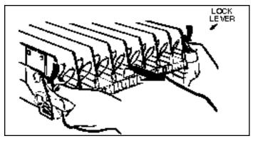
Figure 1. MOVING SHELF TO LOADING POSITION.
