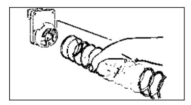
Figure 3. REMOVING AND INSTALLING SPIRAL.
